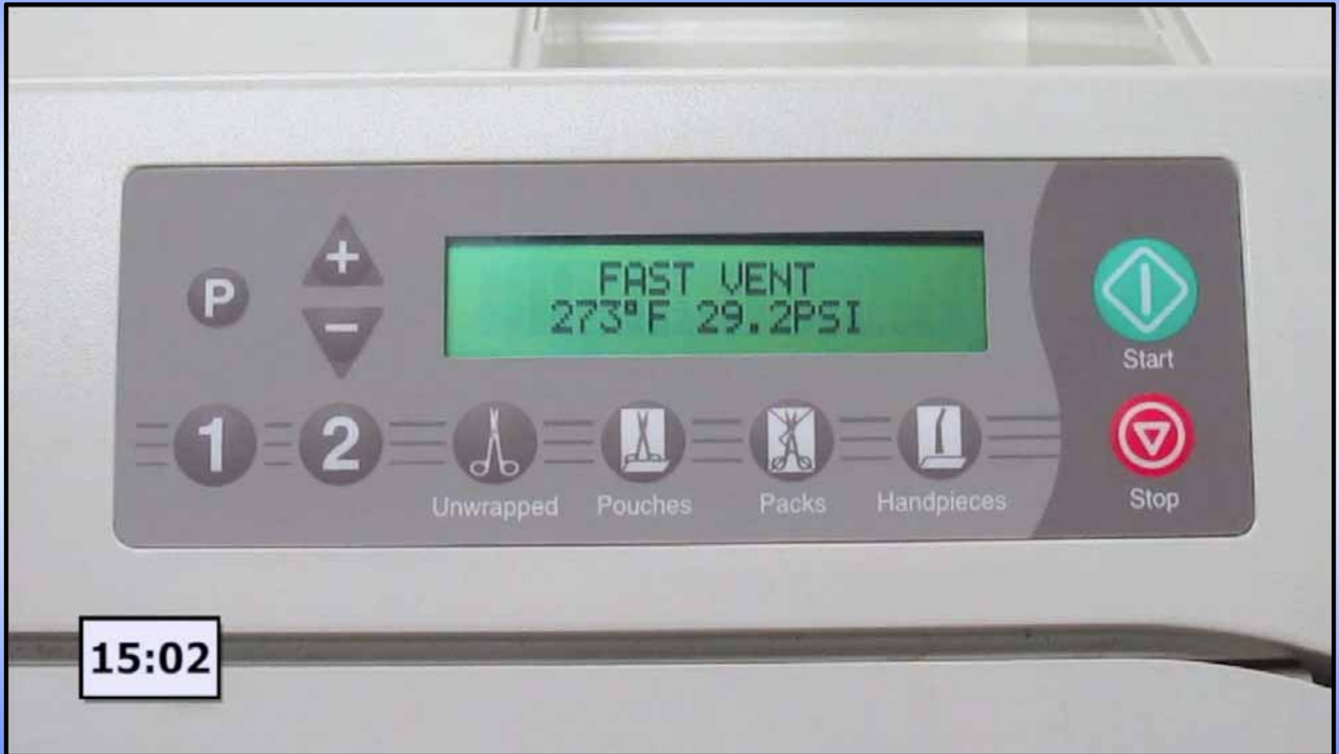
The sound of the Vent Valve opening for the final time signals the beginning of Phase 4.
